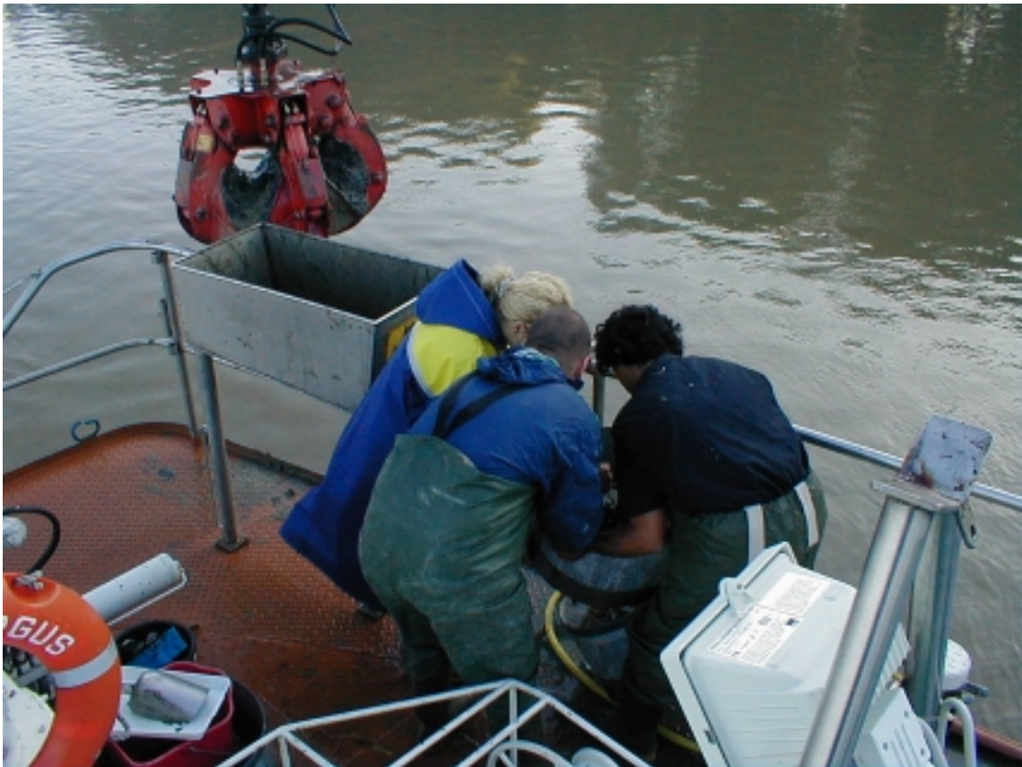
10. Sampling macroinvertebrates by the polyp grab of ARGUS: usually 5 m depth was achieved by that
