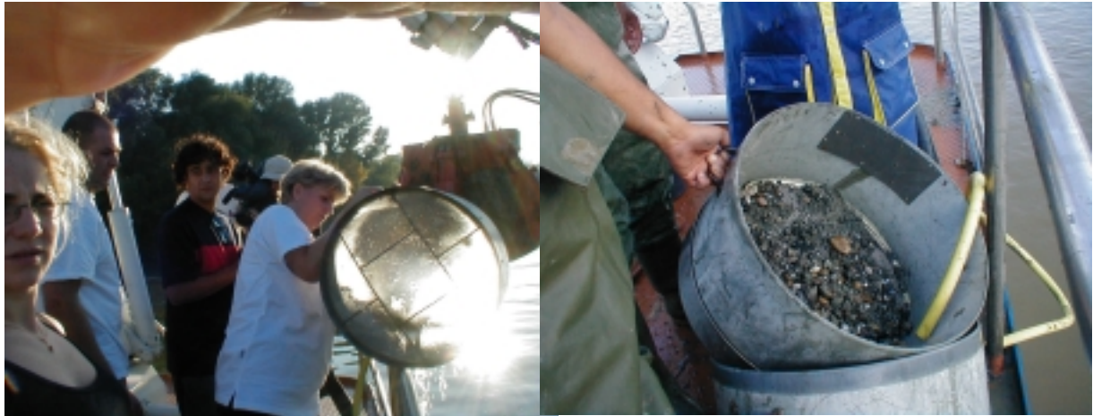
11. Grabbed samples were washed by river water pumped up by the device of the ARGUS laboratory ship
