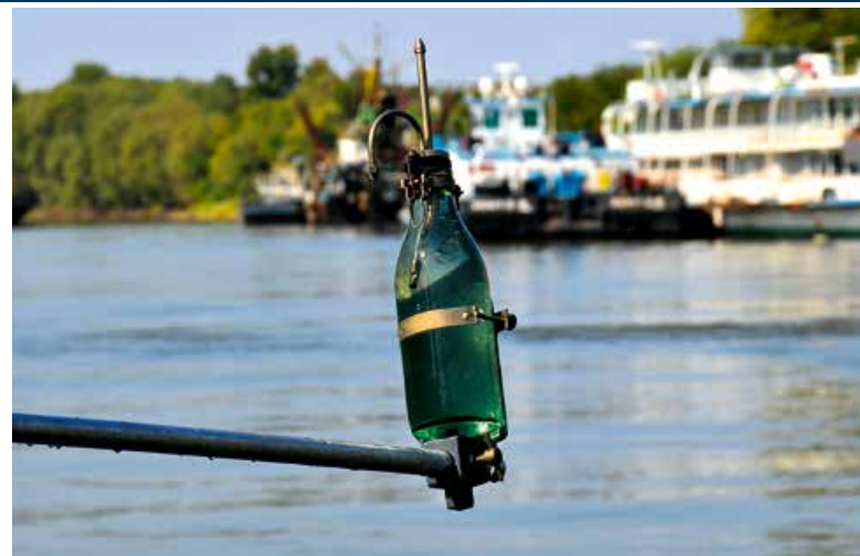
▲ The two photos show instruments used to monitor sediment. The top photo shows a US P63-Sampler, which is a best practice device for monitoring sediment. The photo directly above shows a water sampling method used to analyse suspended sediment. Foto: © Marlene Haimann / IWHW - BOKU
