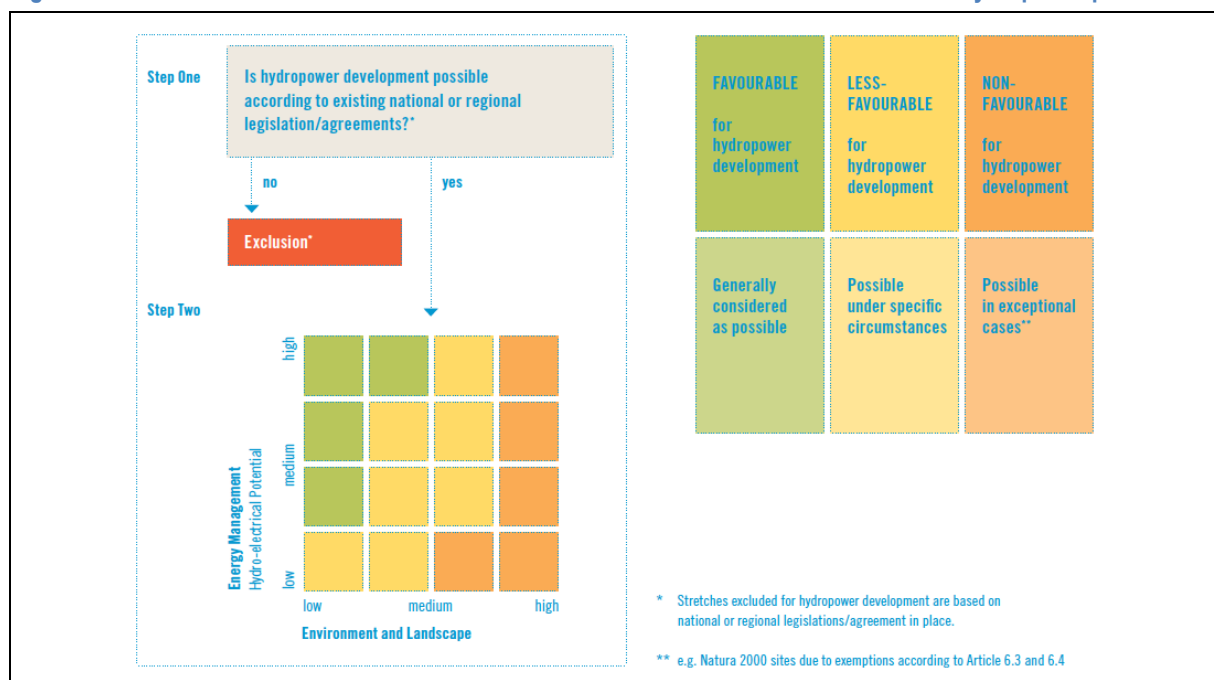
Figure 42: ICPDR assessment matrix and classification scheme to establish the utilisable hydropower potential
